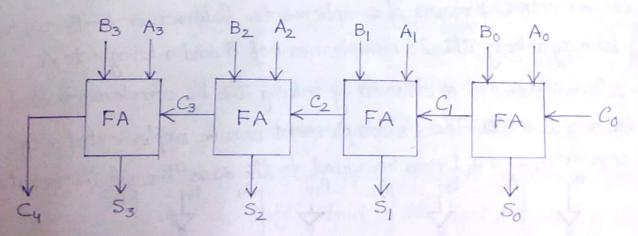
Fig. shows the inter-connection of four full adder (FA) circuits to provide a four-bit binary ripply carry adder. The carries are connected in a chain through the full adders. The Soutputs generate the required sum bits.
