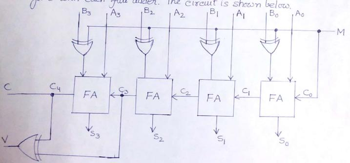
The mode input M controls the operation (adder/subtractor).
